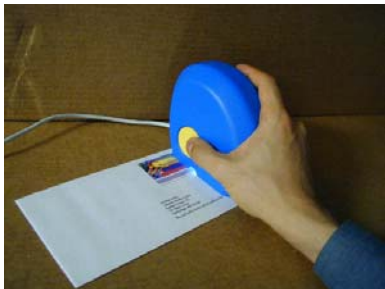
Figure 1. FiberFingerprint verifier for mail piece
