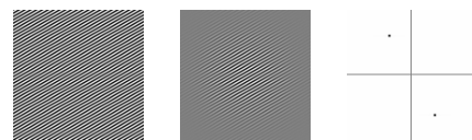
Figure 1 – (From left to right): an elementary component; application of a 2D Hamming window; FFT-based estimation its Fourier magnitude domain.
